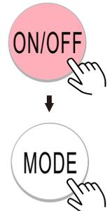
**AUTO** In AUTO operation, the system selects an appropriate operation mode (COOL or HEAT) based on the indoor temperature and starts the operation.
