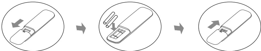
1. Slide to open the battery cover according to the direction indicated by the arrowhead.
