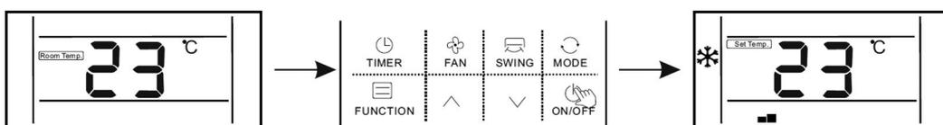
2. When the unit is standby, the wire controller displays indoor ambient temperature (Room temp.), the other content are not displayed.
