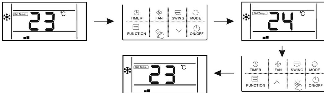
Under COOL, DRY, and HEAT modes, the setting temperature range is 16°C ~ 32°C;
