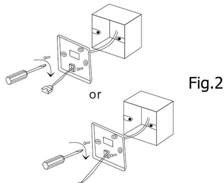
4. After connecting the connecting wire to the main body of the wire controller, as shown in Fig. 3, install main body part according to the following steps:
