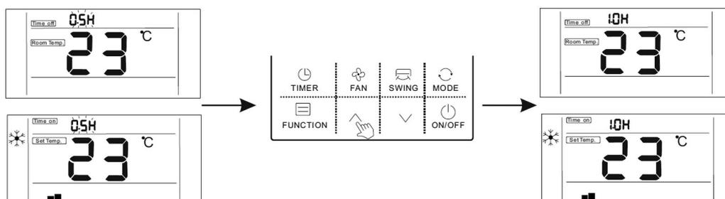
4. After the setting "Timer On" function, you can adjust the fan speed, running mode, set temperature, and swing angle. If there is no operation for 10 seconds, standby screen will be displayed.
