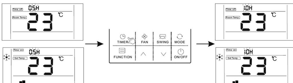
3. After the setting of timing, press "Timer" button again to confirm. The timing setting is successful and the time bar will stop blinking.
