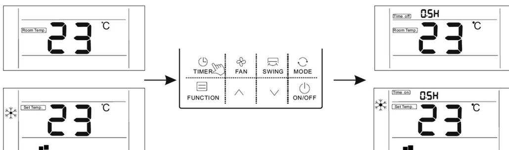
2. After entering timing time setting interface, the default timing time is 0.5H, at this moment, press "▲" or "▼" button to regulate the timing time. If the button is not pressed for 10 seconds, the timing setting will be canceled, and then return to the state of non-timing.
