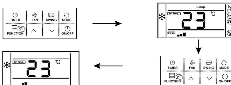
Note: The unit without turbo function can also set turbo function on the wired controller, the performance is high fan speed, but "👉" icon and "Turbo" icon do will not display.
